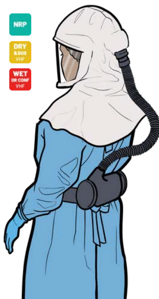
External motor PAPR with hood
