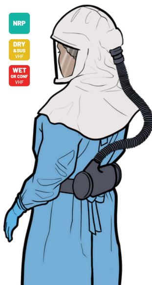
External motor PAPR with hood
